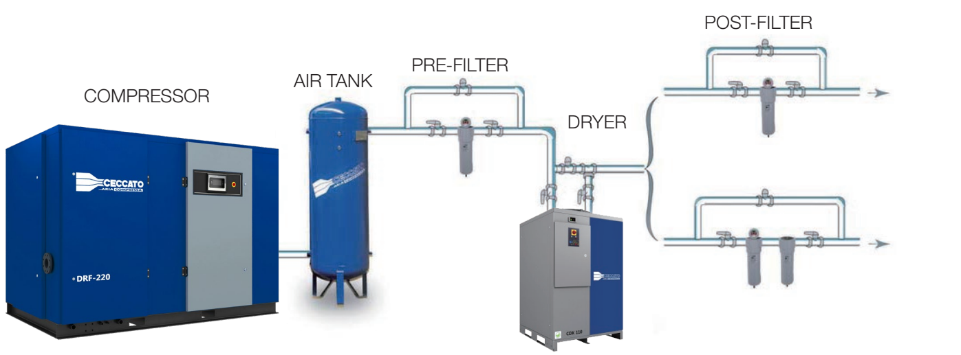
Compressor Station Layout
